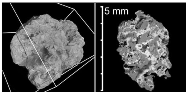
Fig. 1. Example of microtomographic reconstruction. 3D reconstruction of sample 1 (left) and its axial cross-section (right).
