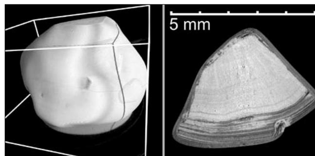
Fig. 2. Example of microtomographic reconstruction. 3D reconstruction of sample 6 (left) and its axial cross-section (right).
