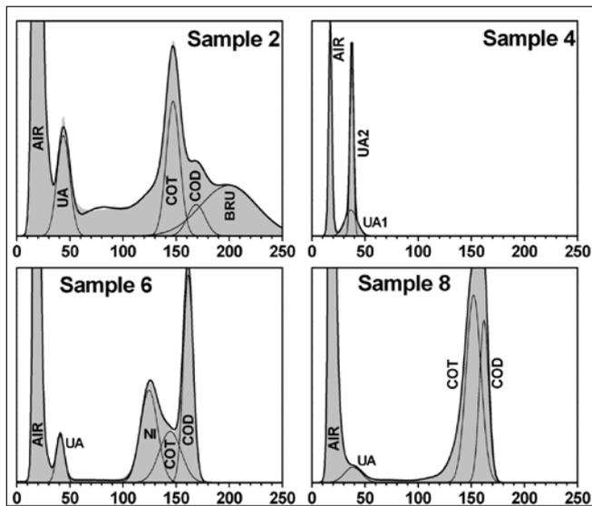
**Fig. 3.** Examples of histogram analysis for samples 2, 4, 6, and 8. The 3D image histograms (grey) were fitted with a set of Gaussian shaped functions. Gaussians drawn with thin lines represent the pattern compounds. The sum of all fitted Gaussians are marked as thick solid lines. COM, COD, and COT – appropriately calcium oxalate mono-, di-, tri-hydrate; BRU – brushite; UA1, UA2 – different uric acid phases; NI – not identified as a pattern component.
